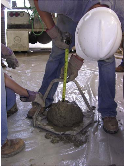
(a) Slump Test
