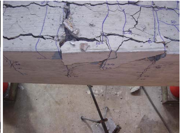
(b) 8-8-2-OC1: Face and Side Split Failure
