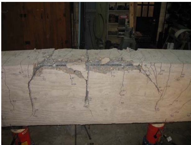
(c) 8-8-3-OC1: Side Split Failure
